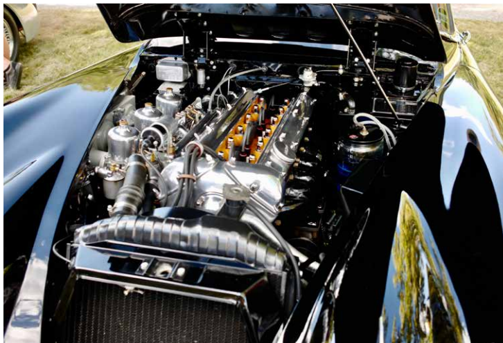
A lovely example of Jaguar's lovely and legendary DOHC in-line six engine
